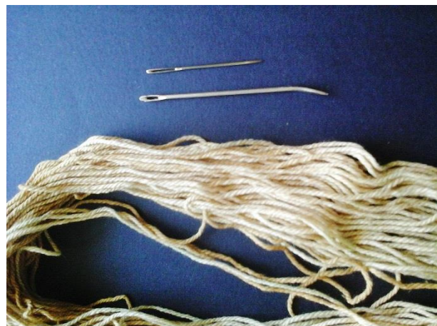
Chenille needle top. Packing needle beneath – generally available from K-Mart, Textile Traders, Spotlight
